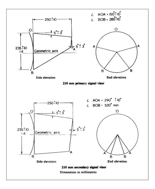
Figure 1 200mm Signal Visor Drawings
