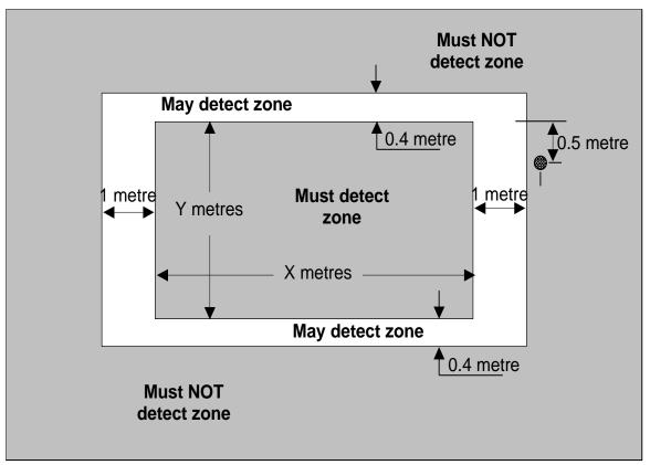
Above Ground Detector mounting pole position
